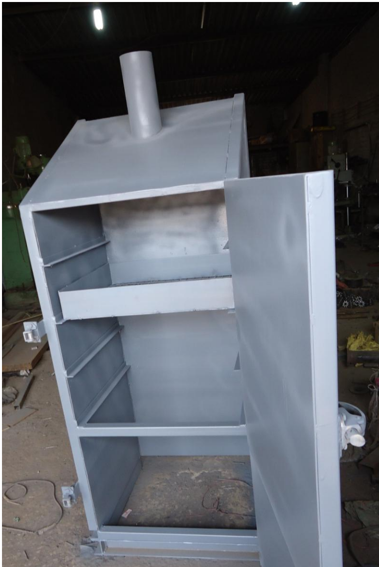
Figure 9: A view of the tender coconut husk dryer
